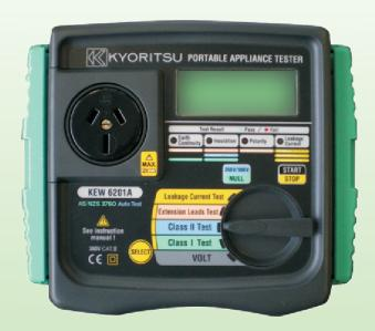
The Model 6201 is a hand-held portable appliance tester, performing four functions to ensure the Safety of Class I, Class II and Class III 240V appliances. And also can measure the mains voltage.
