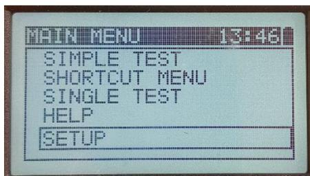
3. Enter SETUP menu using TEST button and move down to COMMUNICATION.
