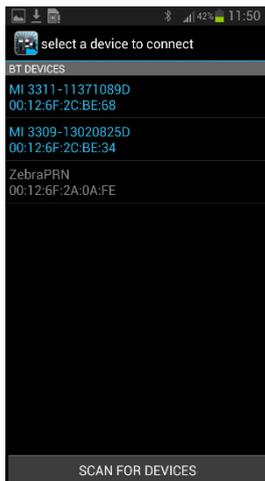
11. As this will be the first time you have connected simply press SCAN FOR DEVICES.
