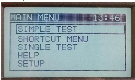
22. Next, select the type of test you want to perform using the up/down keys, for this example we will use an IEC cord.
