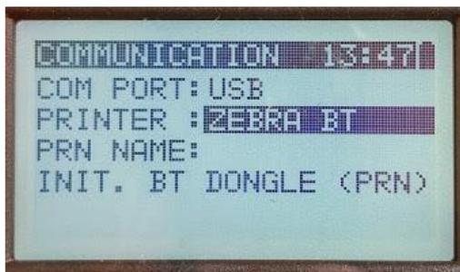
6. A list of available BT devices will be displayed. Select printer ZebraPRN and press TEST button to confirm. It should now Say PRN NAME: ZEBRAPRN
