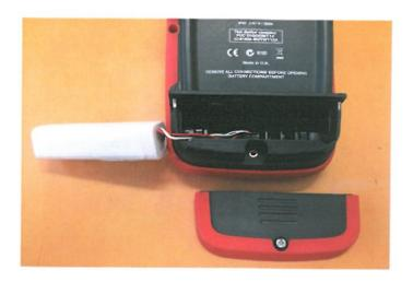
3: Lift rear cover off unit and fold to one side, as per photo, this will expose the 2 mains fuses.
