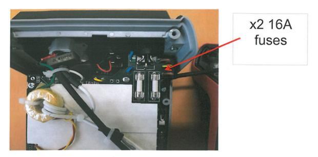
5: Reassemble in reverse order. Be carefull of camera cable when reassembling.
