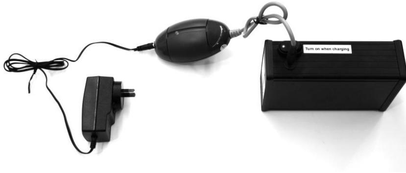
Plug the transformer into the battery and the wall adaptor into the wall power outlet; ensure that the battery is turned on while charging. There should be an LED illuminated on both the transformer and wall adaptor.
