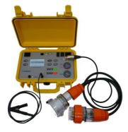
**Set up:** Select the appropriate 1 or 3 phase test lead and insert control plug into utility socket as shown in picture.
