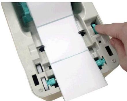
Hold the Top cover and press the top cover support to disengage the top cover support with lower inner cover. Gently close the top cover. Make sure the cover latches securely. →
