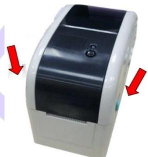
← Separate the media holders to the label roll width.
