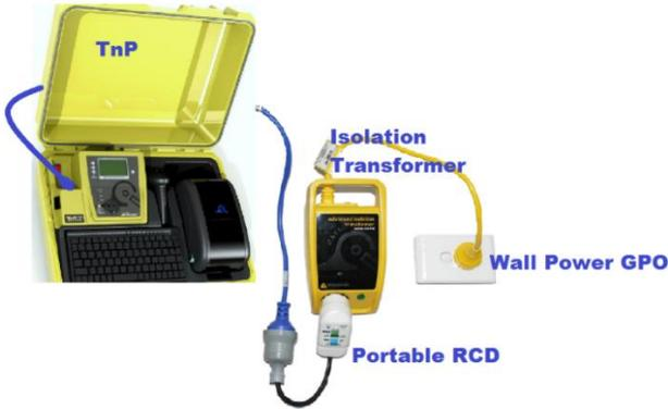
Diagram 2 For Testing Fixed RCD -All models
