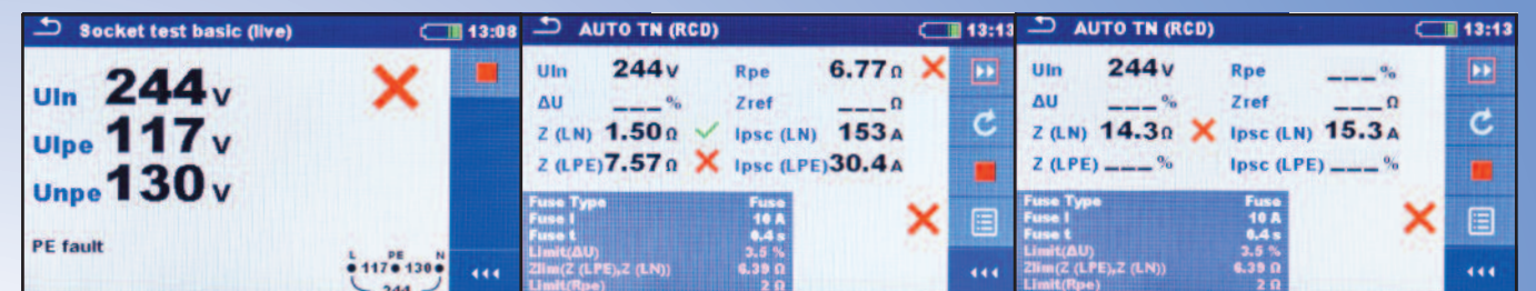
Earth Open Circuit FAIL Result
